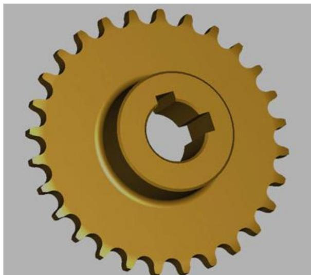
**Picture No. 9-** Execution of two keyways on gear for chains
