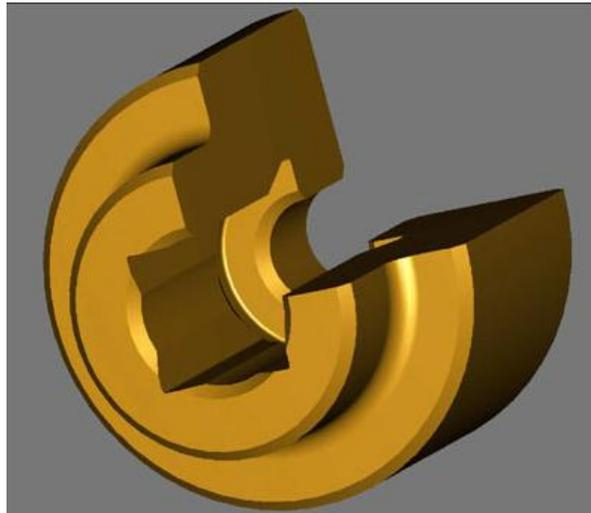
**Picture No.10-** Execution of an internal square connection on a hub
