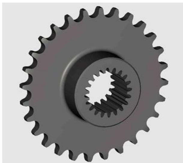
**Picture No.11-** Execution of internal gear teeth on a gear for chains
