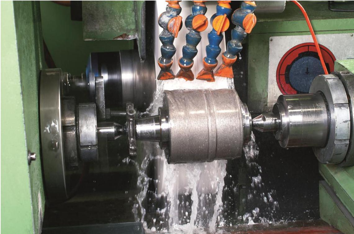
**Figure N°3** – Dressing operation with a diamond roller
