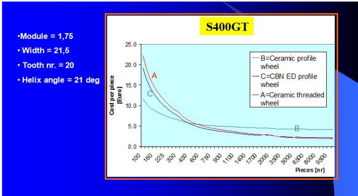
Fig.N°7- Cost comparison per piece between the different grinding methods
