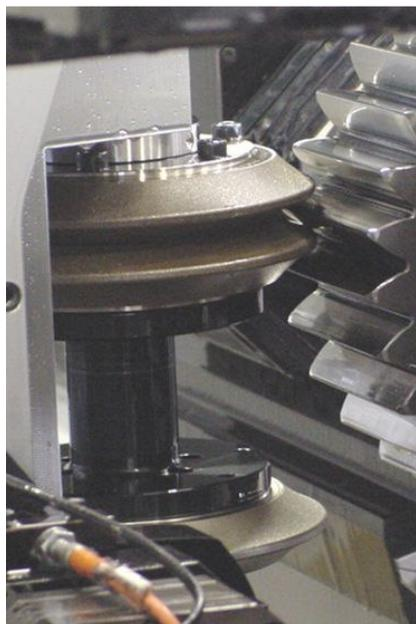
**Fig:N°2-** Profile grinding with a electroplated CBN form wheel
