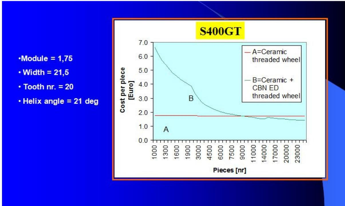
Fig.N°6- Cost comparison per piece between the different grinding methods
