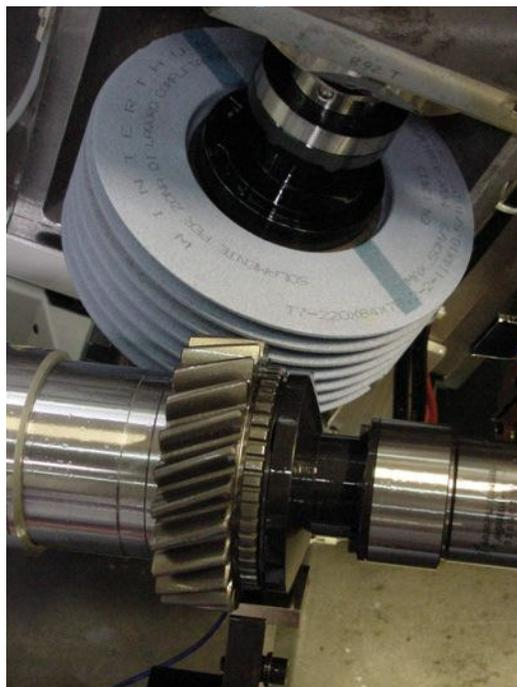
**Fig. N°1-** Continuous generating grinding with a worm ceramic wheel
