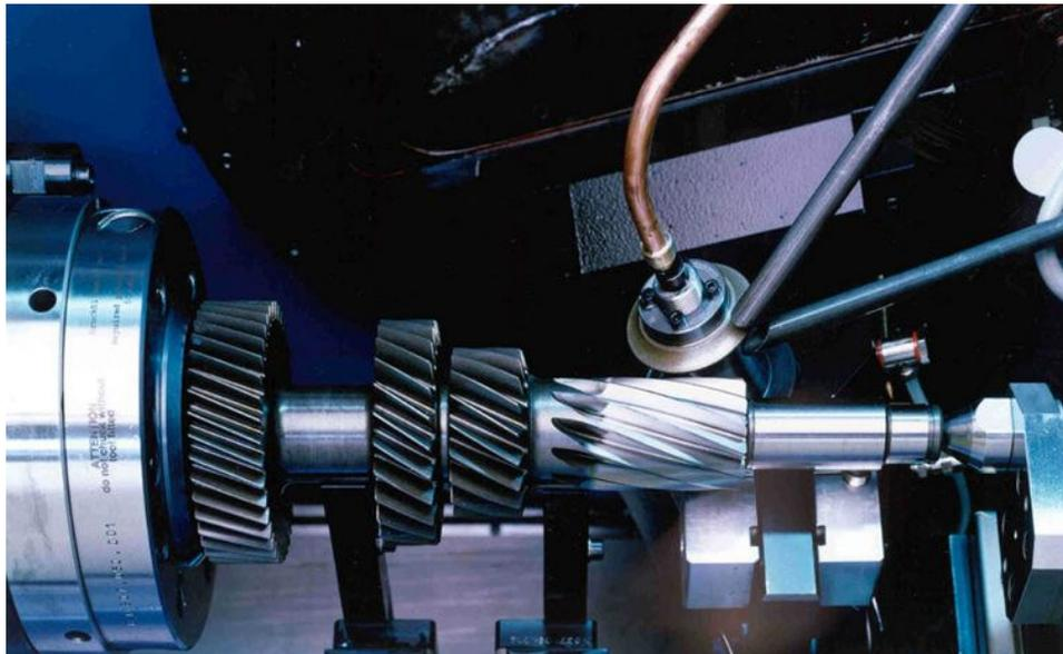
**Fig.N 3-** With a small diameter form wheel it is possible to grind gears close to a shoulder
