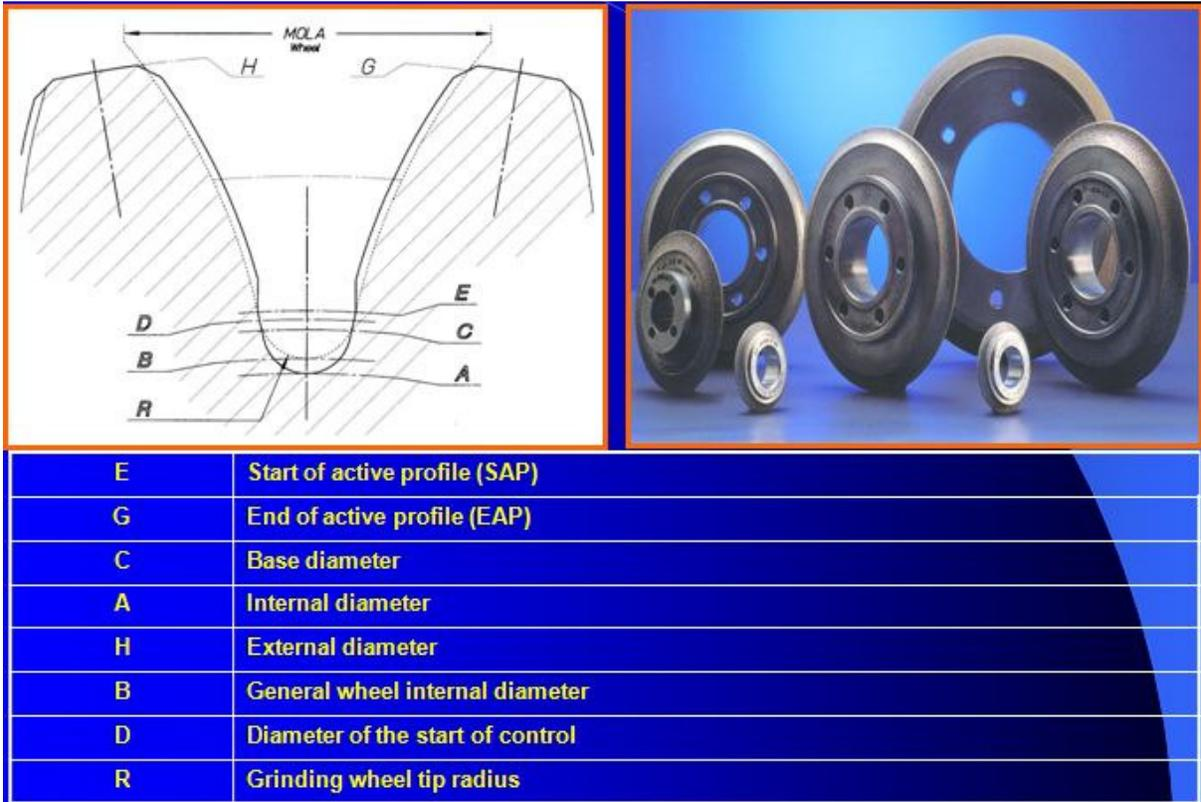
**Fig. N°4-** Form wheels are able to grind along the whole tooth profile
