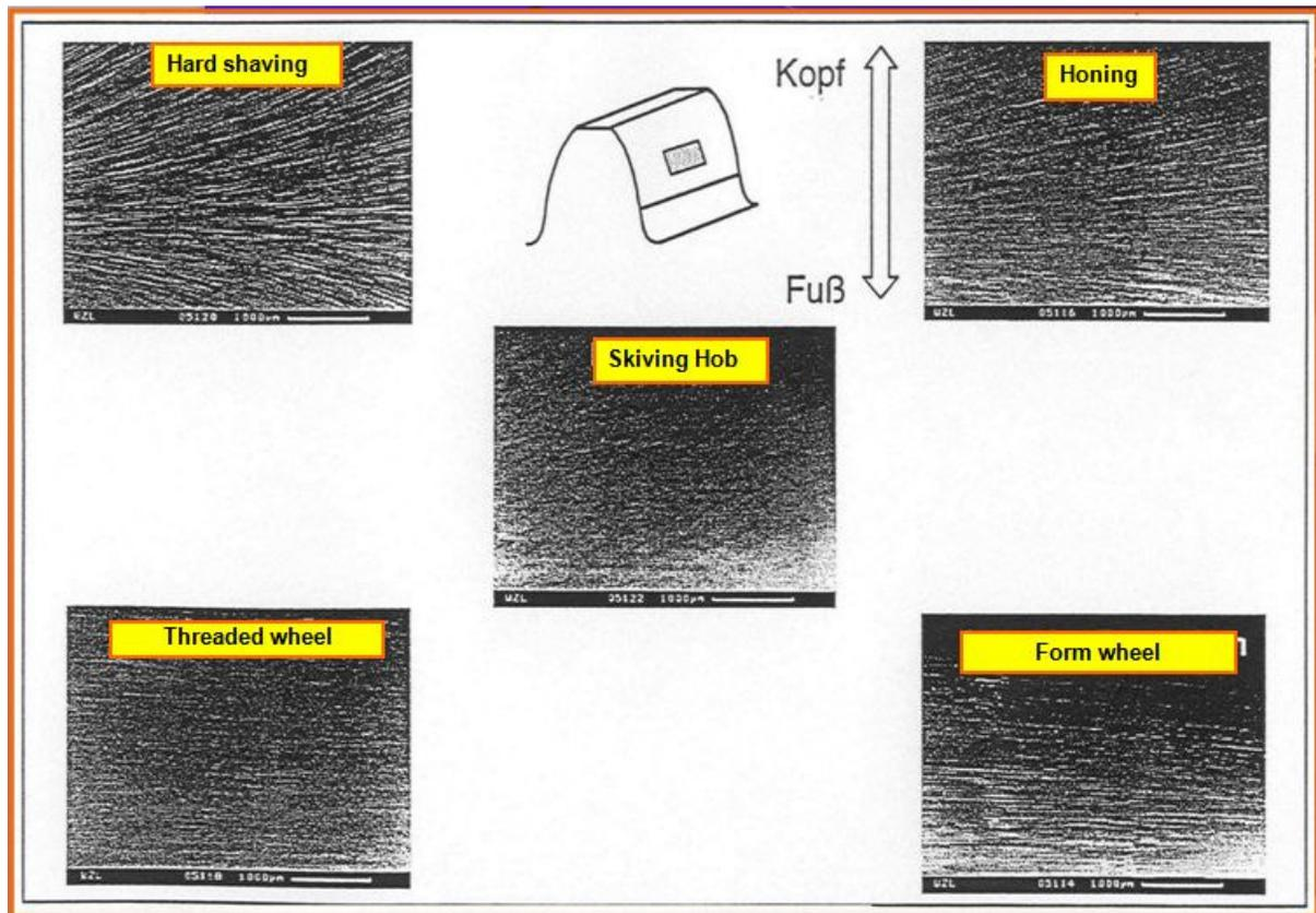
**Fig. N°5-** Comparison between surface quality obtained with the different finishing methods
