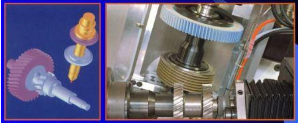
**Fig. N°6-** *Combination of two different types of form wheel for high precision grinding of two different gears and combination of a CBN worm wheel and a ceramic honing tool*
