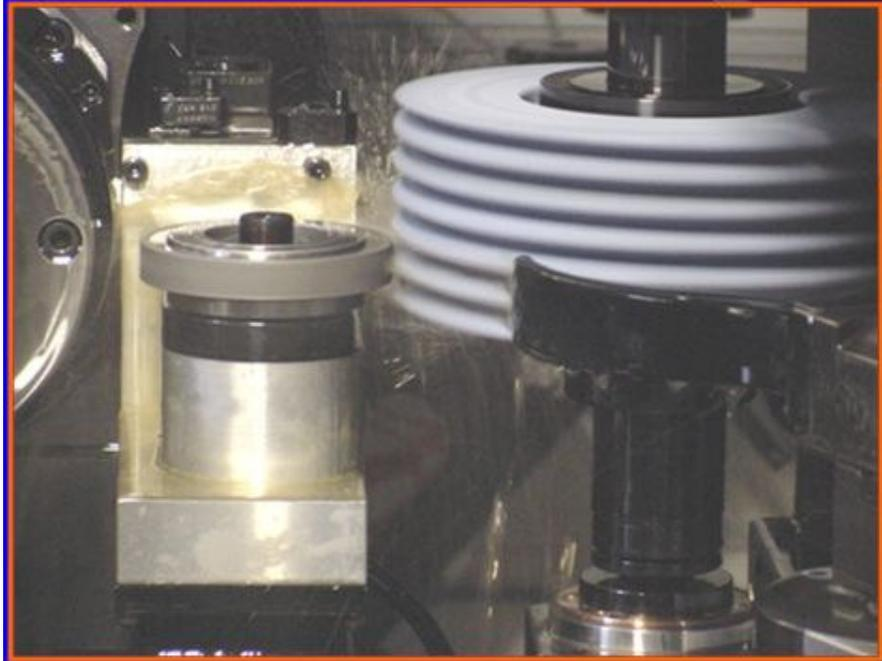
**Fig. N°8-** *Diamond dressing of worm wheel external diameter*
