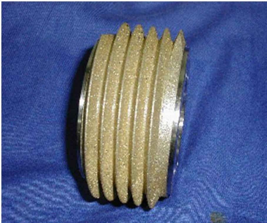
**Fig. N°3-** *Electroplated CBN worm grinding wheel*
