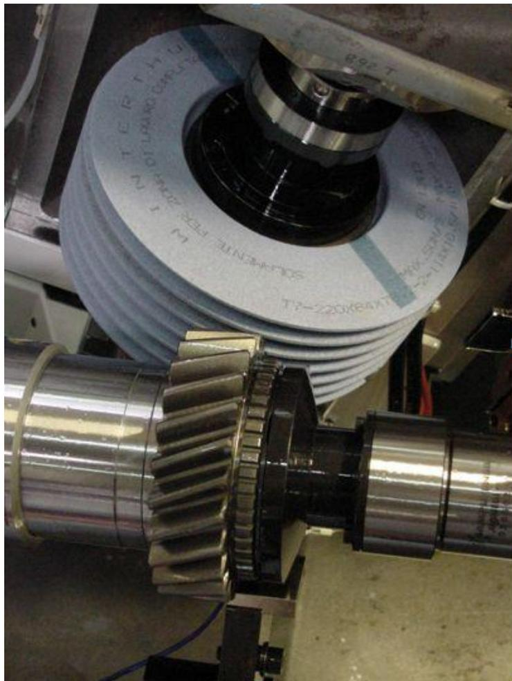
**Fig. N°1** – *Grinding with worm wheel*
