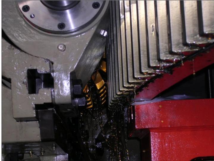
**Figure N°1**- *Hobbing of a big gear*
