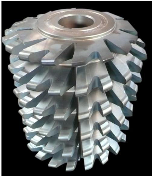
**Figure N°3-** Hob with roughing and finishing teeth
