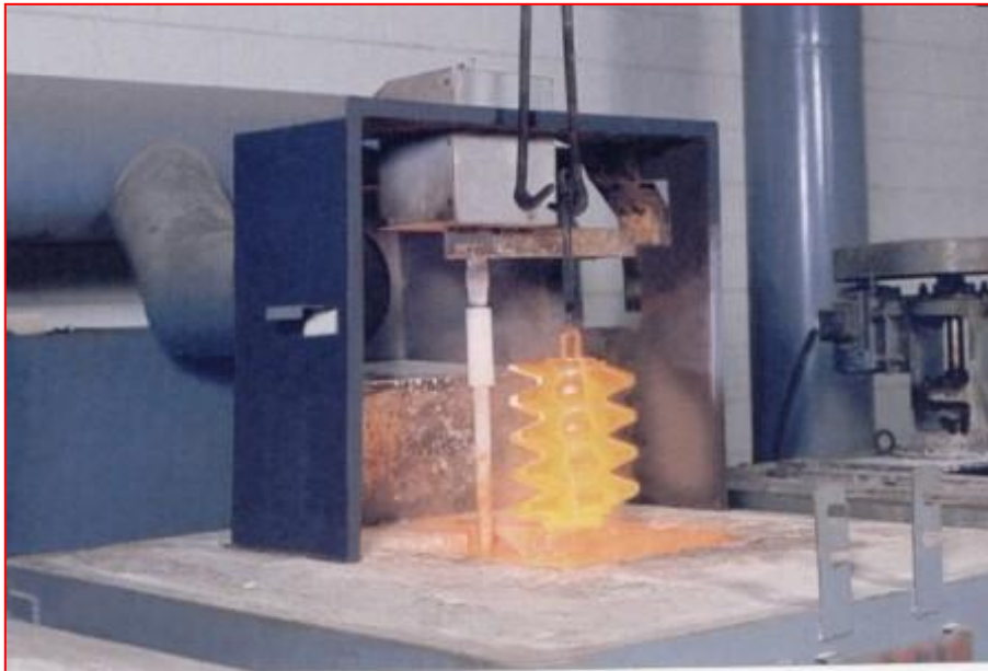
Figure N°1 – Heat treatment of a hob.
