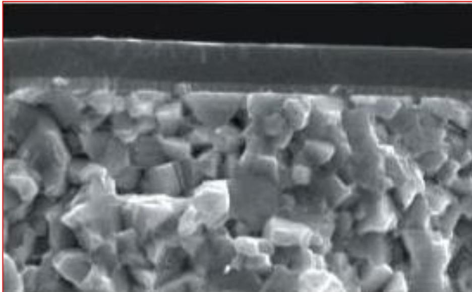
**Figure N°1-** DLC coating on sintered carbide (Korloy – Corea)
