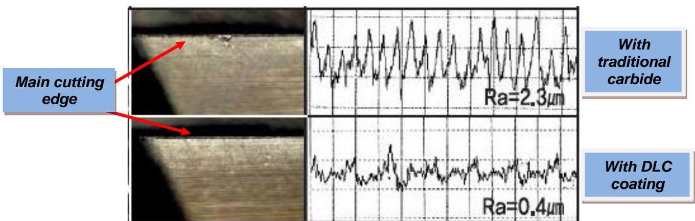
**Figure N°4-** Example of reduction of surface roughness using DLC coatings
