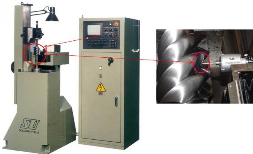
Figure N°5- Checking equipment linked with grinding machine
