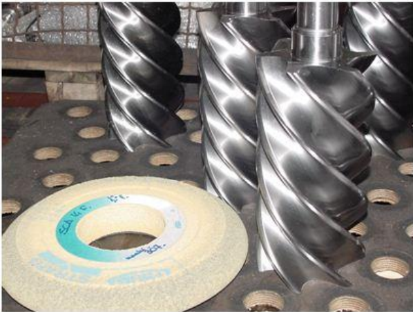
Figure N°3- Both ceramic and CBN wheels can be used
