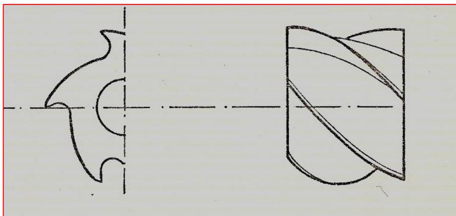
**Fig. N°3-** Milling cutters type T
