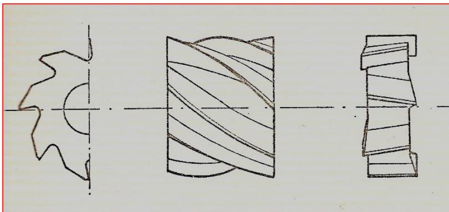
**Fig. N°1-** Milling cutters type N
