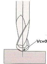
*The better tilt is at 15° in the feed direction and allow the mill to work to a cutting speed equal to 80% of the maximum theoretical one in reference to the nominal diameter of the cutter itself.*
