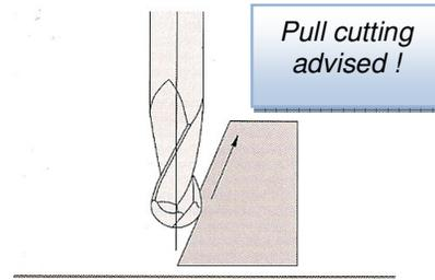
*Concordant milling gives a better quality result than discordant milling: better surface roughness, less noise, and longer tool life.*
