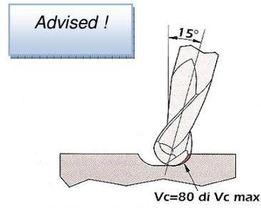
*Do not carry out vertical movements of immersion in the piece, we recommend spiral or ramp movements.*
