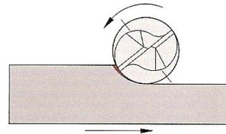
*If possible the tools should be slightly tilted in the feed direction to avoid any working in the central part of the tool where the cutting speed is equal to zero.*
