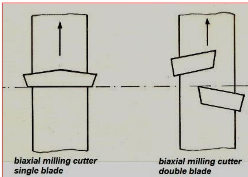
**Fig. N°3-** Milling cutter with bi-negative inclination of the cutting edges
