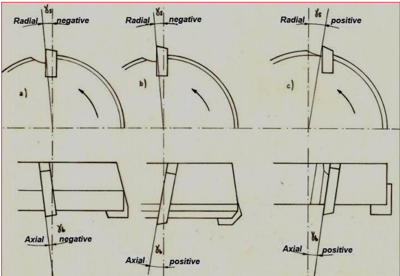
Fig. N°1- Schematic indication of the various combination of the typical angles
