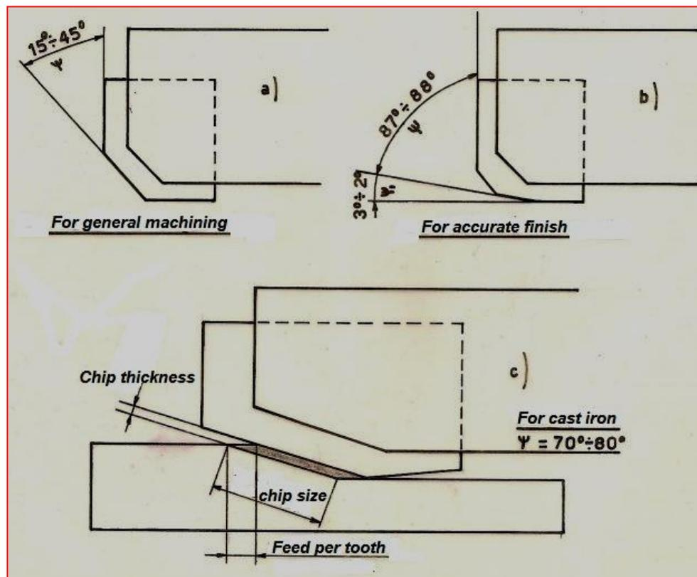
**Fig. N°2-** Different angles of peripheral cutting edge
