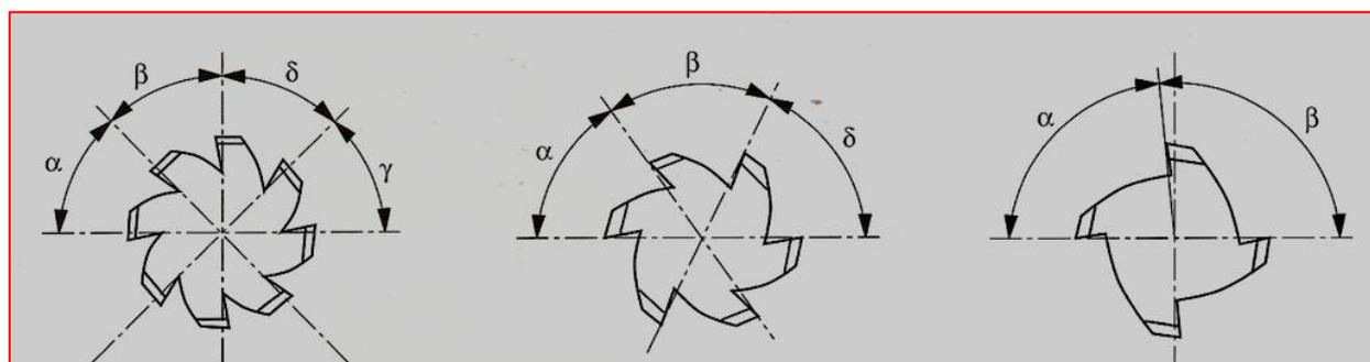
**Figure N°1-** *Irregular division of the cutting edges to prevent vibrations*
