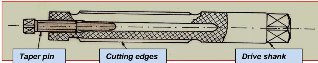
**Figure N°2-** *Expandable reamer for through holes (manual)*
