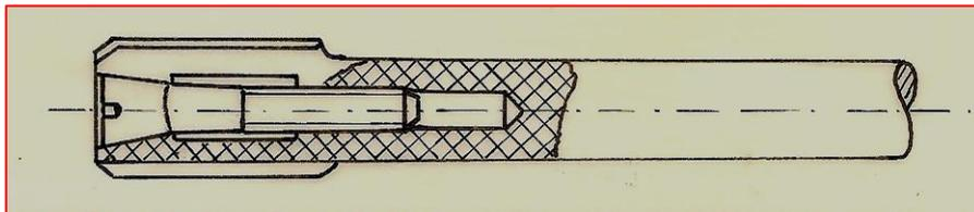
**Figure N° 3 -** *Expandable reamer for blind holes (usable on machine tools)*
