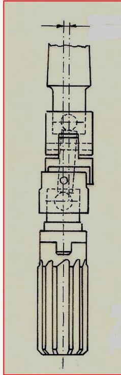
**Figure N°6-** *Oscillating assembly for reamers*
