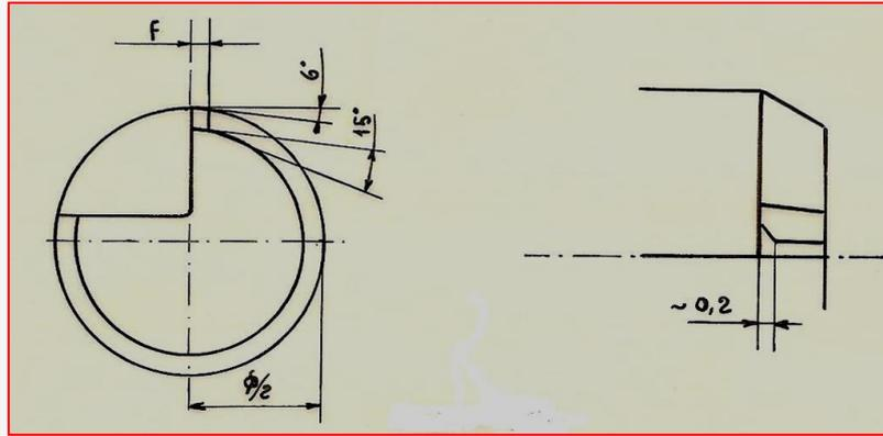
**Figure N°7** - Rake angles of a single cutting edge reamer
