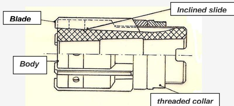
**Figure N°5-** Adjustable blade reamers sleeve type
