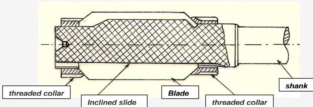
**Figure N°4-** Adjustable blade reamers shank type
