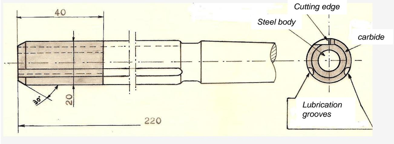
**Figure N°8-** Single cutting edge reamer
