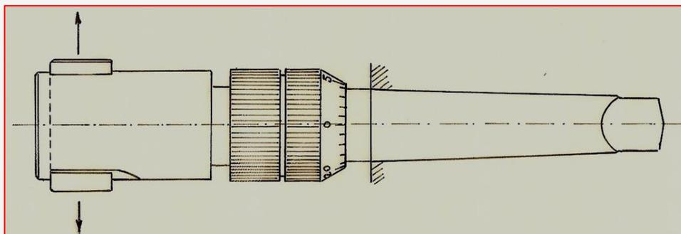
**Figure N°6 –** *Oscillating reamer*
