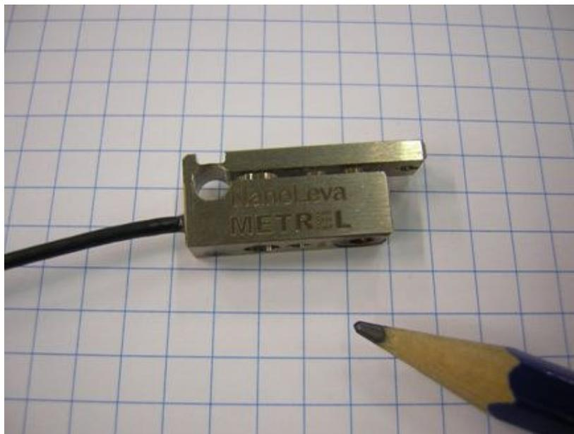
**Figure No. 3-** *Small transducer called NanoLeva*
