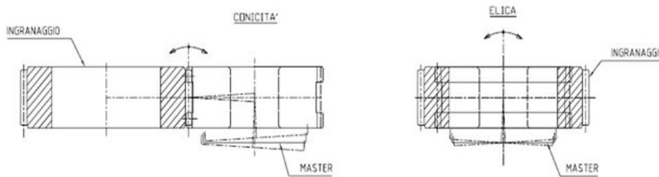
**Figure No. 6a-** *Diagram of master floating movements for control of helix*
