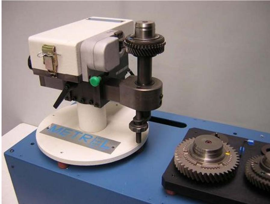
**Fig. No. 1-** *Equipment for control of OBD dimension*
