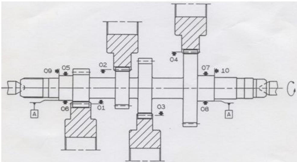
**Fig.No.8-** Measuring diagram of a shaft with 4 tooting.
