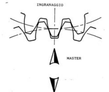
**Figure No. 5-** Operating principle of rolling gear tester at zero clearance
