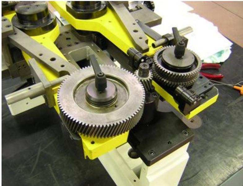
**Figure No. 6b-** *Application of a carriage and special master for control of helix*
