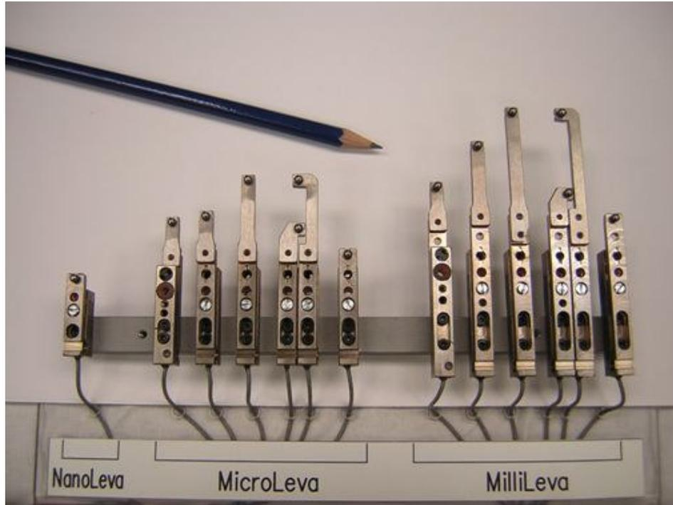
**Figure No. 4-** Selection of different transducers types
