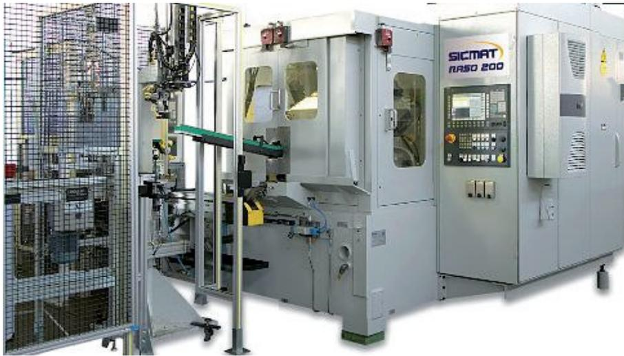
**Fig. N°4** – *Shaving machine RASO 2300 CNC with auto loading system*
