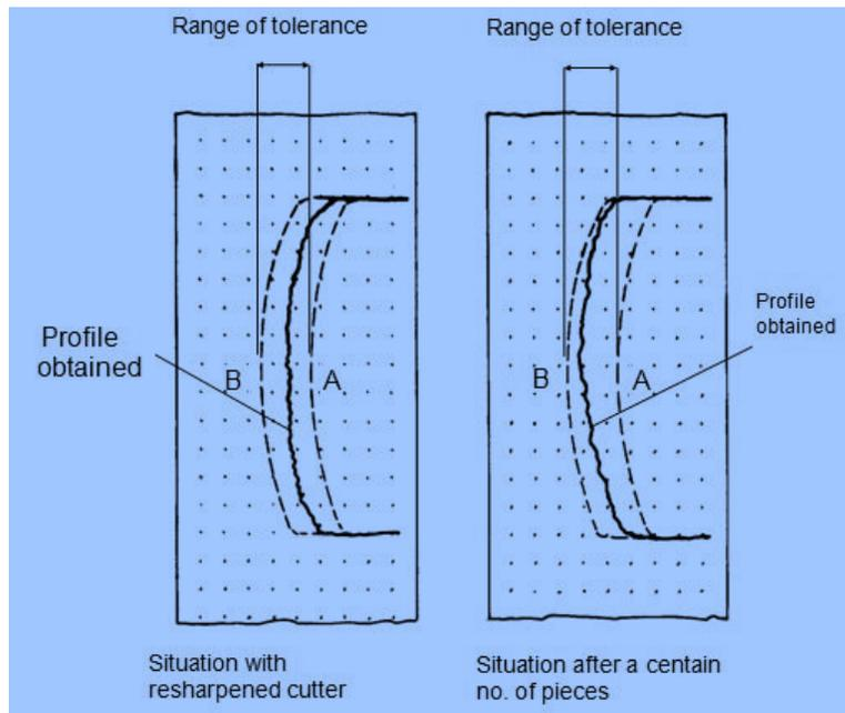
**Fig.N°1-** Profile variation according to shaving cutter wear
