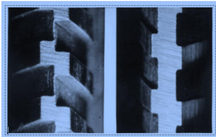
**Fig.N° 59-** *Serration conditions at beginning and end of life*
