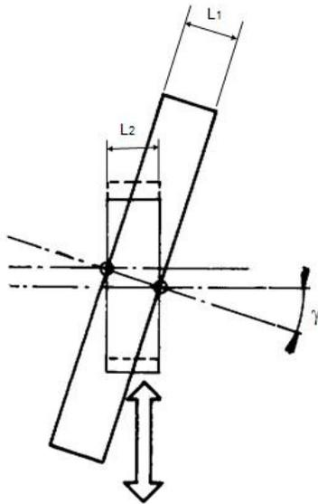
**Fig.N°4-** Underpass shaving scheme ( $\gamma$  = cross of axes angle)
