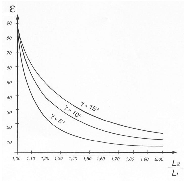
**Fig.N°3-** Correspondence between the maximum diagonal axes and the ratio  $\frac{L_2}{L_1}$  for cross of axes angles of  $5^\circ$ ,  $10^\circ$  and  $15^\circ$
