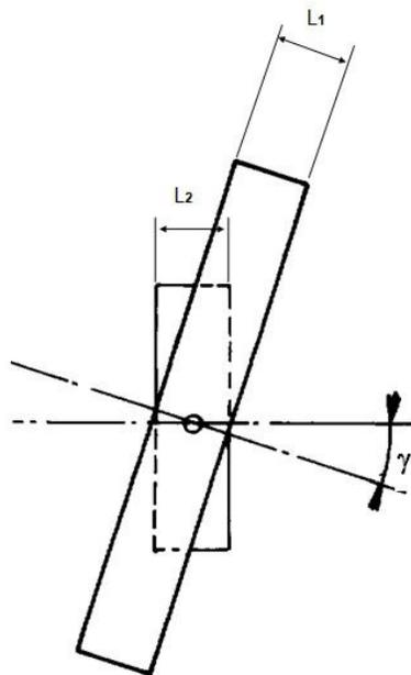
**Fig.5- Plunge shaving scheme ( $\gamma$  = cross of axes angle)**
