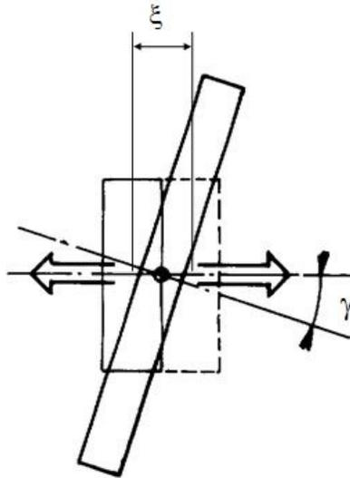
**Fig.N°1-** Parallel shaving scheme ( $\gamma =$  cross of axes angle)
