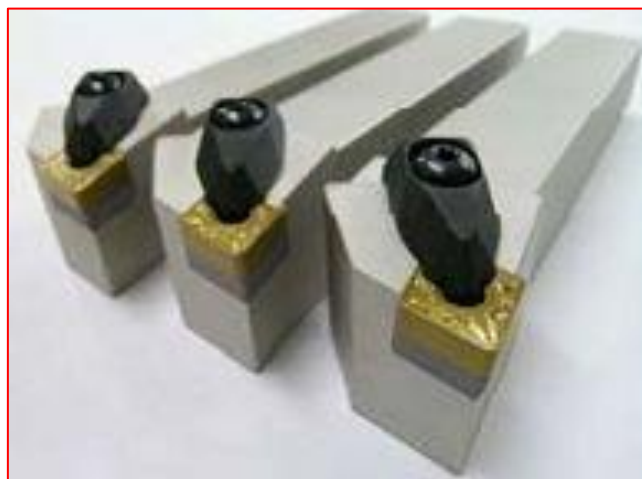
Figure # 2 - Examples of tools named indexable inserts (inserts mechanically clamped)
