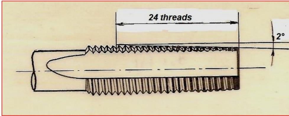
**Fig. N°5-** Extra-Long chamfer for nuts
