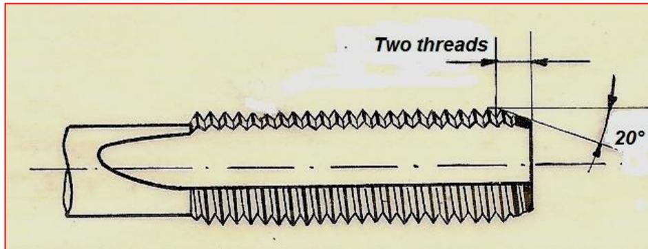
**Fig.N°3-** Modified chamfer for blind holes
