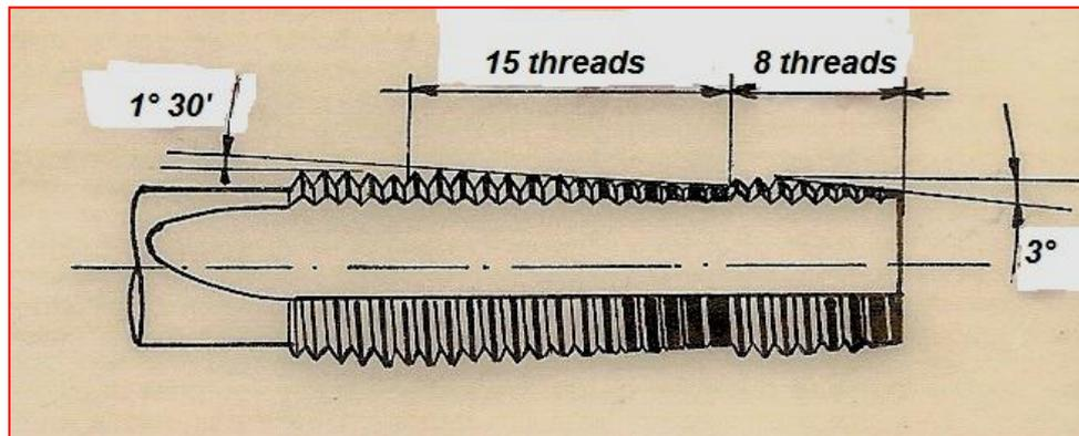
**Fig. N°6-** Extra-Long chamfer for nuts with roughing sector
