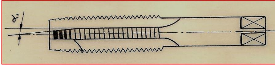
**Figure N°2** - Schematic representation of corrected chamfer, used for long-chipping materials and through holes or blind holes with large room at the end of the hole.
