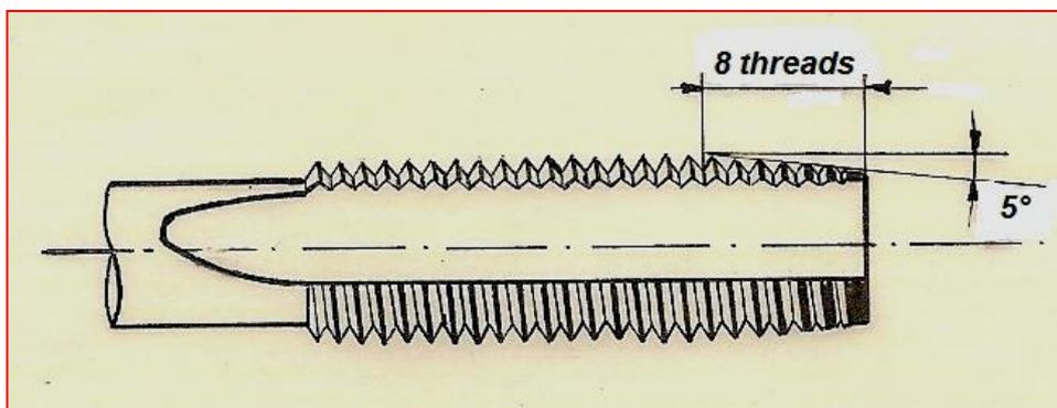
**Fig. N°4-** Long chamfer for not blind holes
