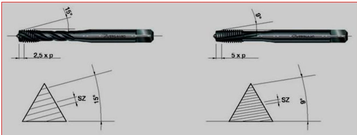
**Fig. N°1** – Difference of the chip thickness in the case of two entrances with different inclinations (Vergnano – Chieri - Torino)
